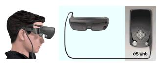
eSight uses breakthrough technology to capture, enhance, and display a real-time video that enables sight for people with low vision and legal blindness. eSight is hands-free, mobile, and multi-use, which means that users can move seamlessly between activities.
